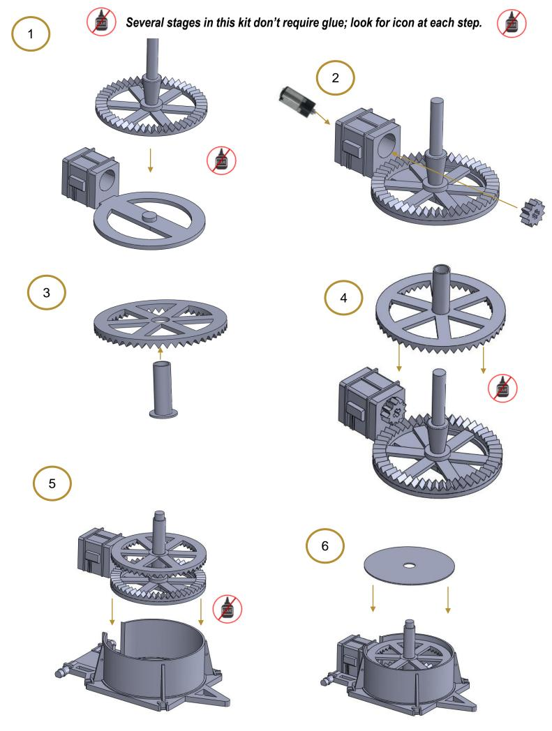
Test run mechanism before securing lid
